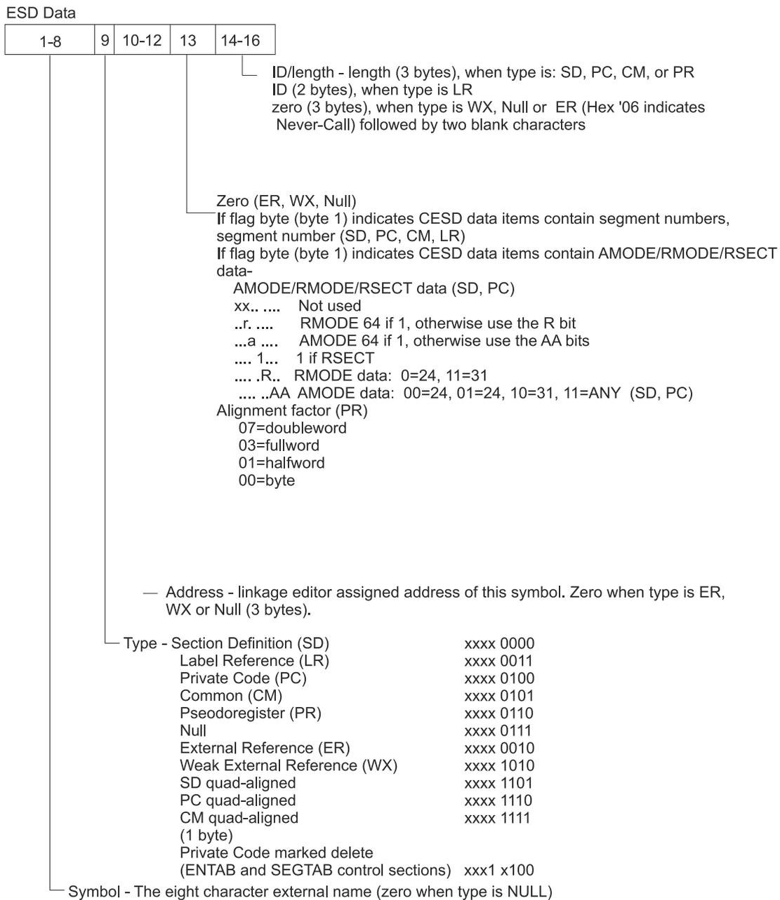
Figure 2. CESD record (load module)
